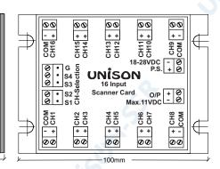
Scanning for 16 Input CH1 TO CH16
